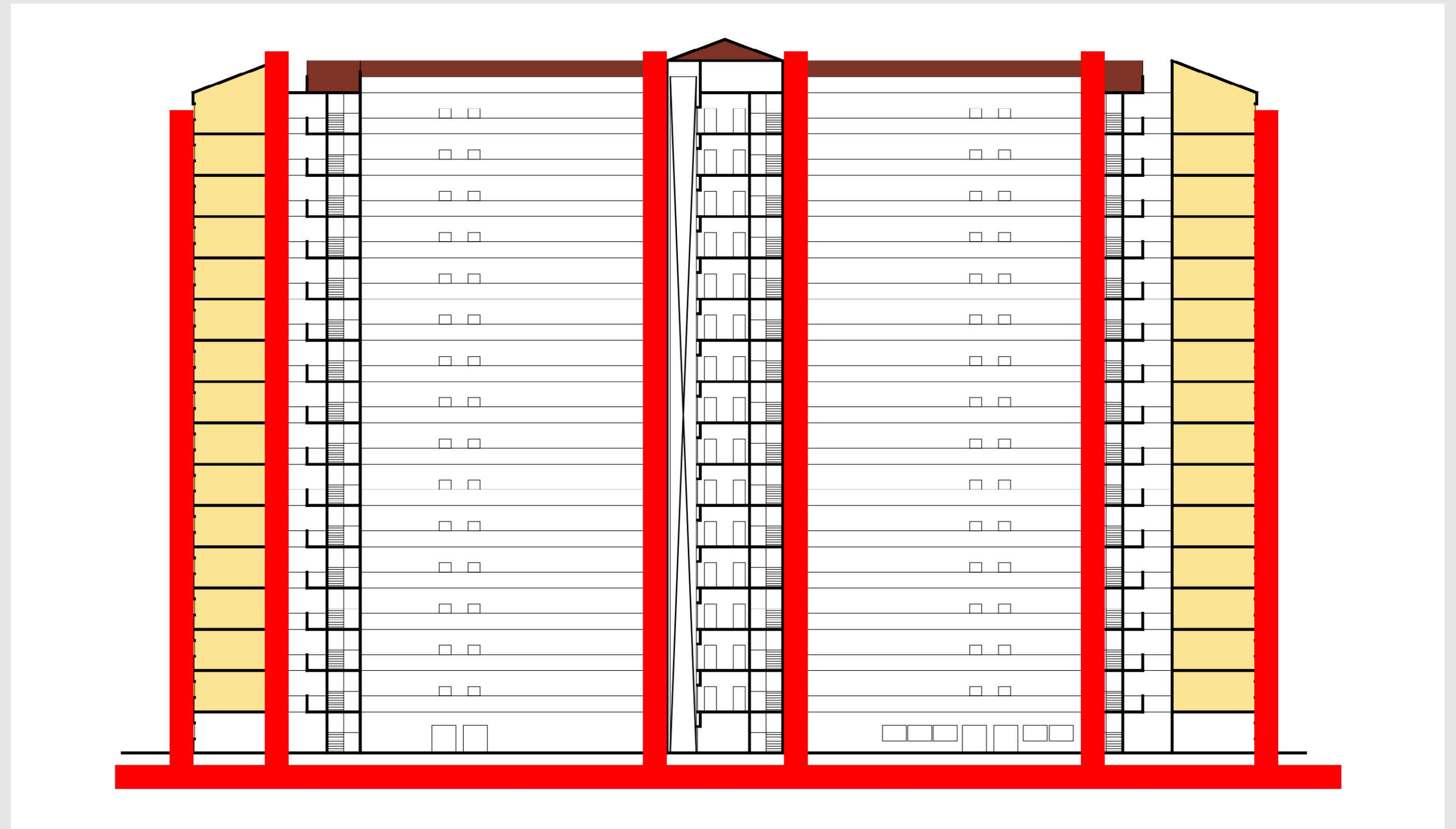
Cross-section of rain gutters and inter-floor drainage within the block (Source: Think City)
